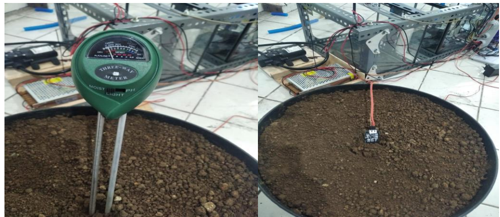
Figure 6. Comparison of soil moisture measurement using a soil moisture meter and a soil moisture sensor
