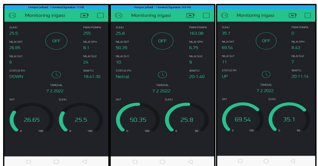
Figure 10. Soil Moisture, Temperature and PWM Readings of the Blynk Application Pump
